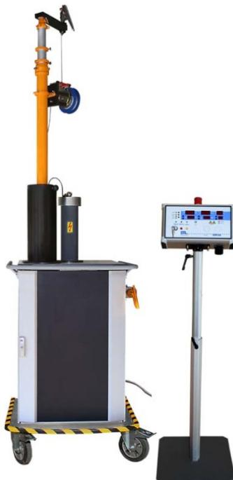
The telescope mast will be integrated into the power unit of the test system.
